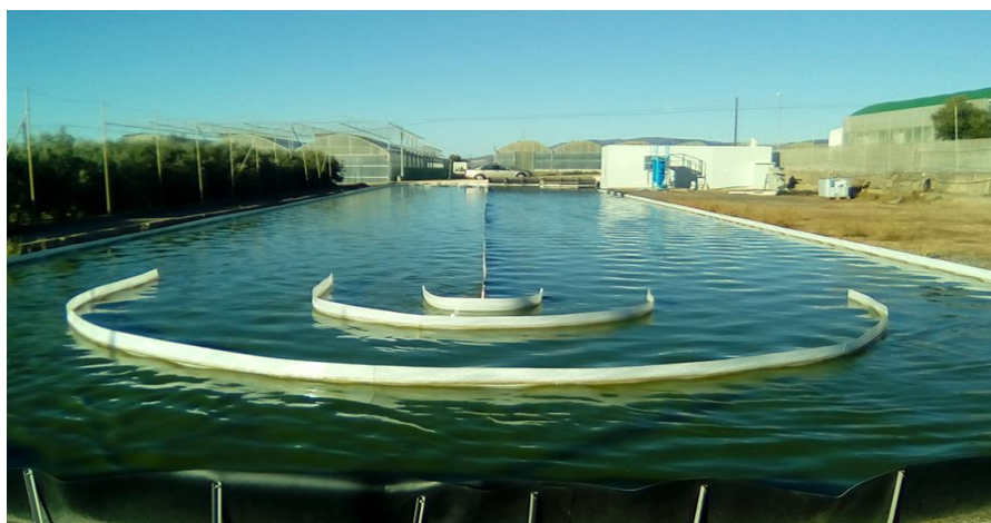
Raceway reactors for microalgae biomass production located at the IFAPA facilities near the UAL campus.
