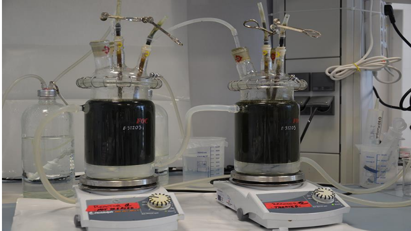
Bench-scale anaerobic digesters located at the IMDEA-energy facilities.
