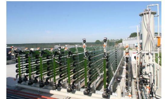
Horizontal tubular PBR 0.56 m 3
