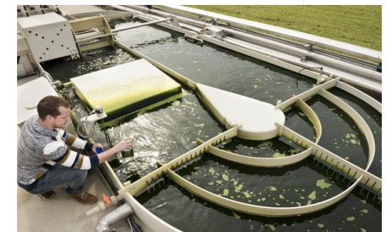
Horizontal tubular PBR 0.56 m 3
