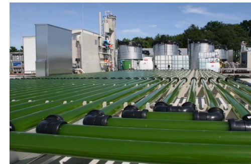
Vertical tubular PBR 0.56 m 3
